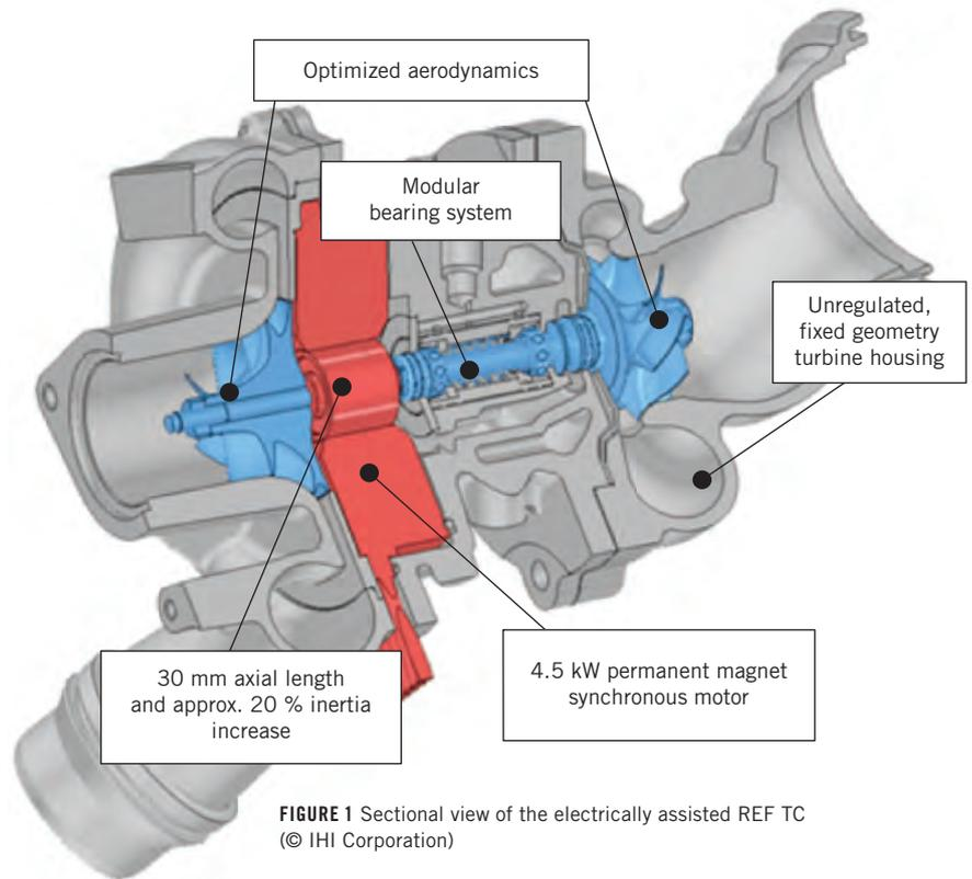
**FIGURE 1** Sectional view of the electrically assisted REF TC
