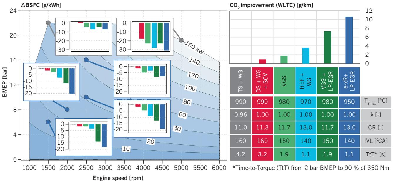
FIGURE 3 Results of ΔBSFC and CO<sub>2</sub> reduction in the WLTC and optimized engine parameters (© IHI Corporation)
