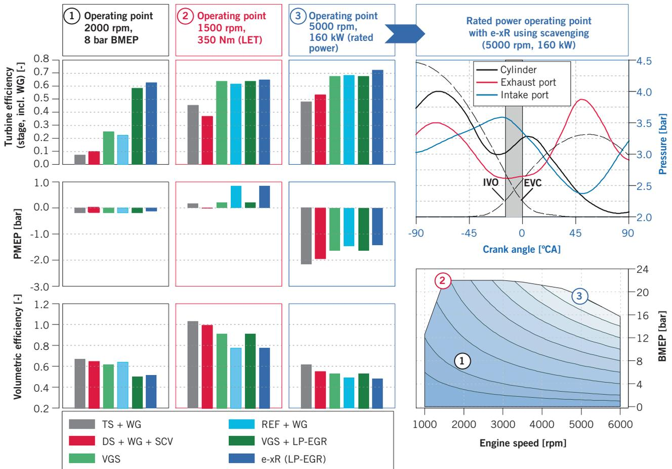
FIGURE 4 Engine gas exchange parameters (© IHI Corporation)
