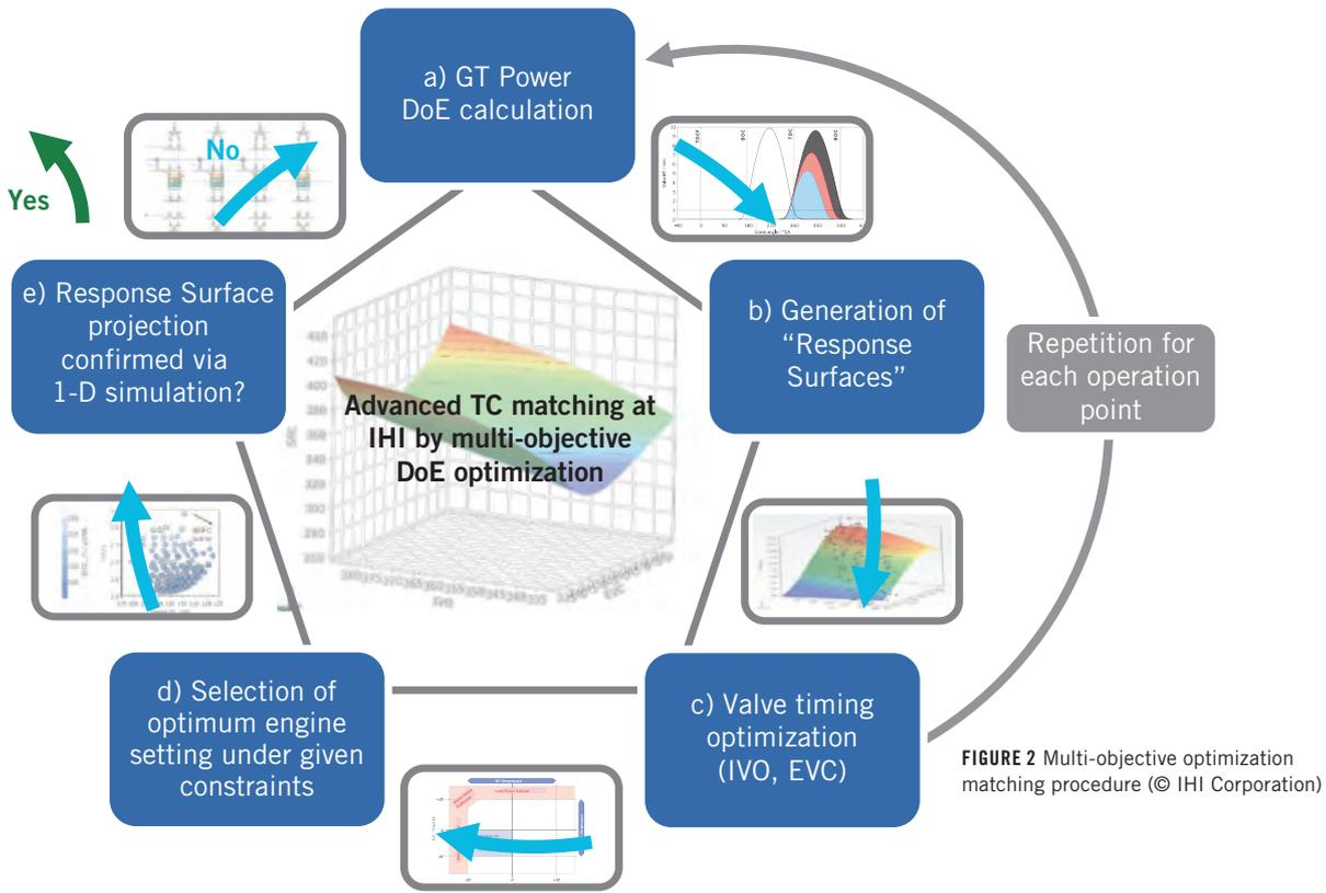
FIGURE 2 Multi-objective optimization matching procedure (© IHI Corporation)
